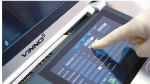
Super-sensitive touchscreen allows smooth operation even with gloves on
